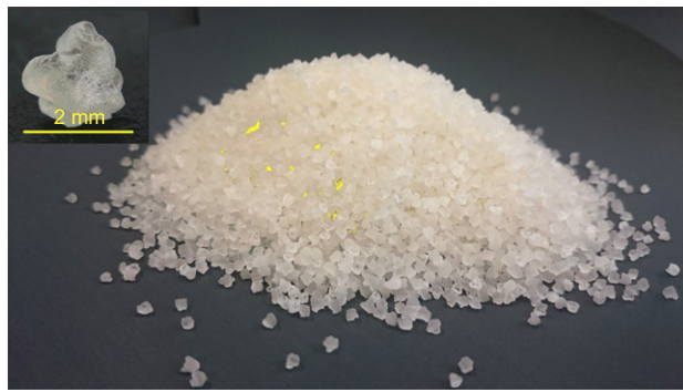
Fig. 10. Bulk printed granular material with inset showing rough angular particle
