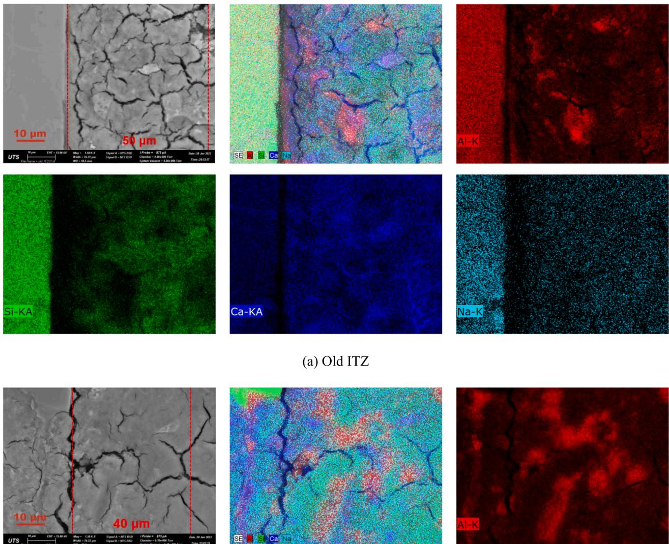
Fig. 9. EDS mapping analysis of ITZs.
