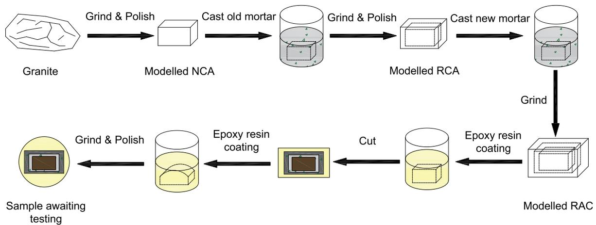
Fig. 3. Process of MRAC sample preparation.
