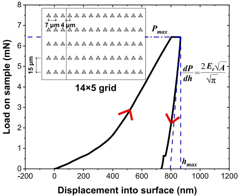
Fig. 5. Grid nanoindentation and a typical load-depth curve.
