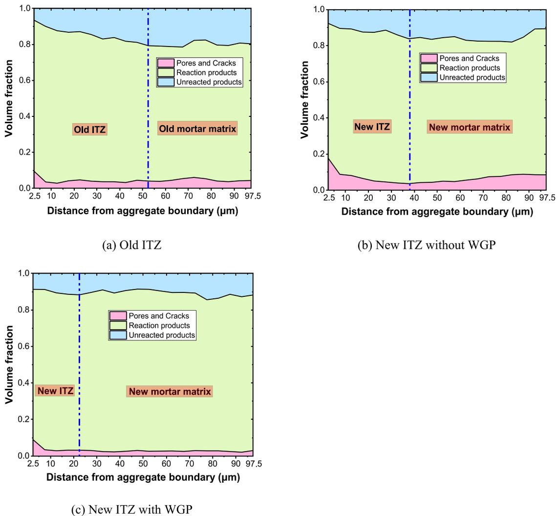
Fig. 8. Phases volume fraction from aggregate boundary to the mortar matrix.
