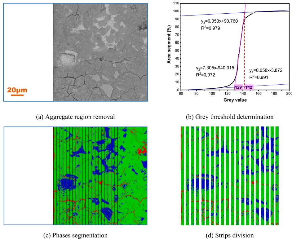
Fig. 7. Schematic view of BSE image processing.
