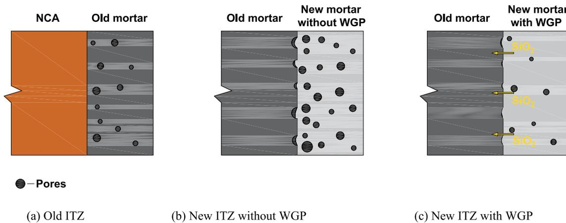
Fig. 15. ITZs microstructure general view and WGP enhancement mechanism.
