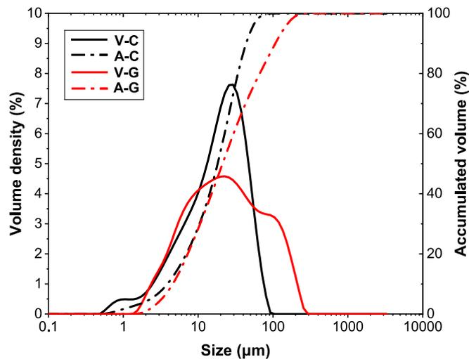
Fig. 2. Particle size distribution of cementitious materials tested by Master-sizer 3000.
