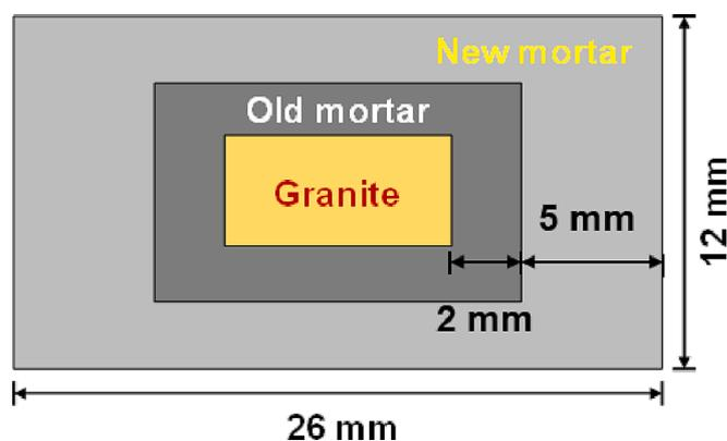
Fig. 1. Schematic diagram of MRAC.
