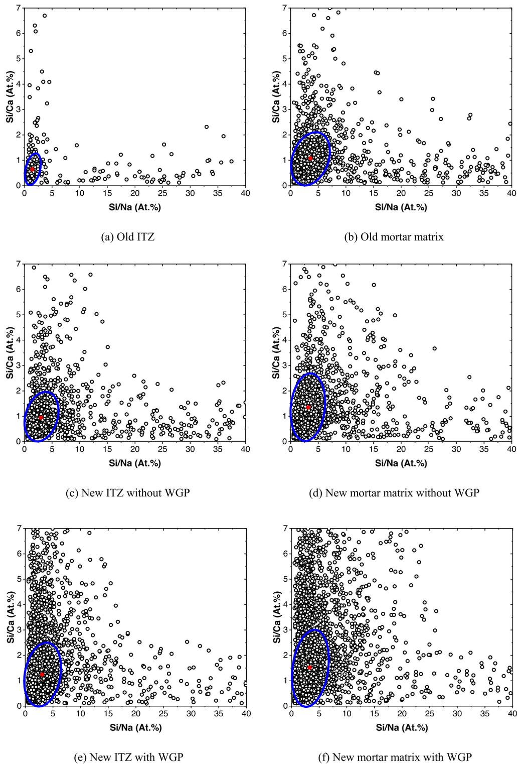
Fig. 10. Atomic proportions of element statistical results in ITZs and mortar matrix.
