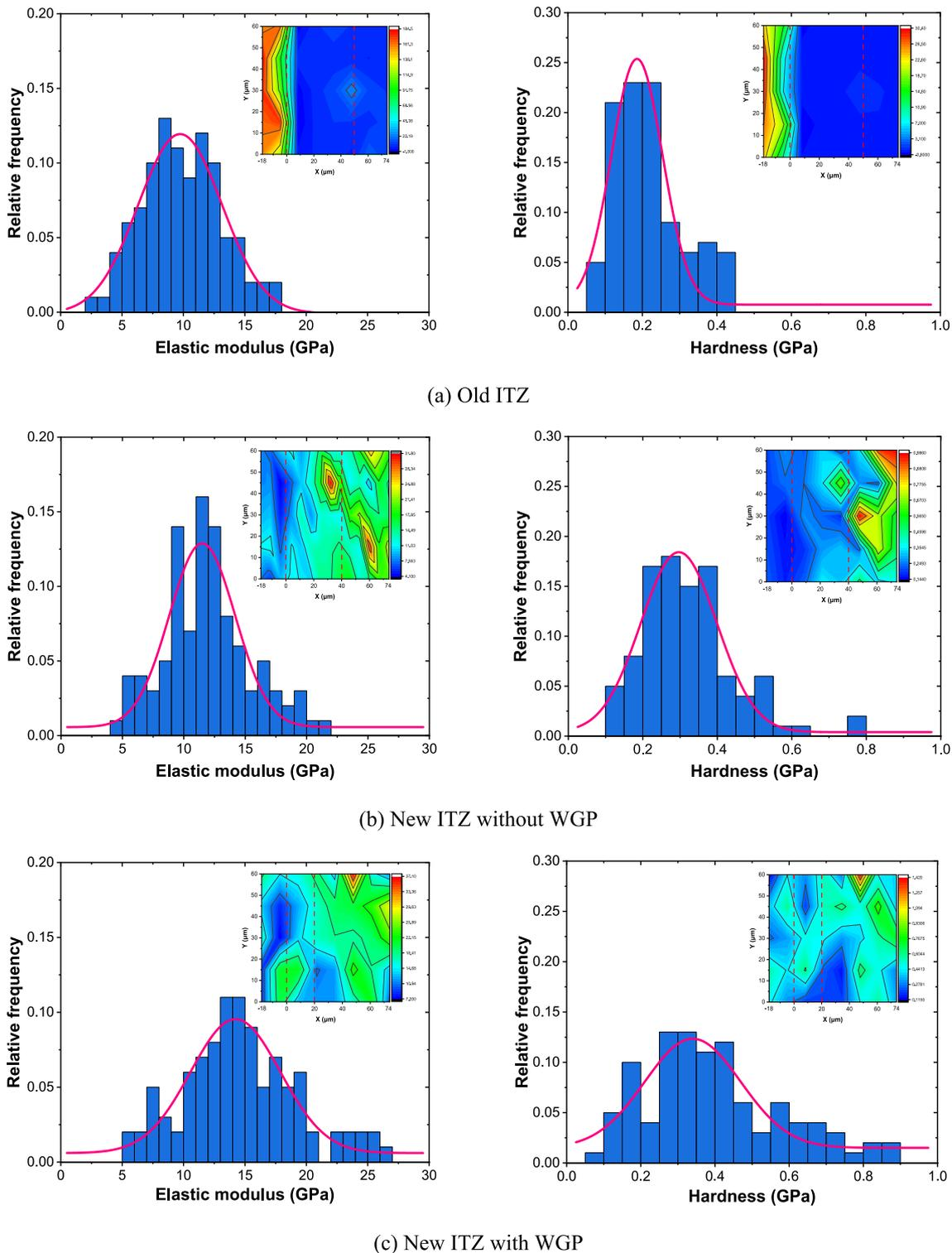
Fig. 14. Distribution of grid nanoindentation results in modelled ITZs.
