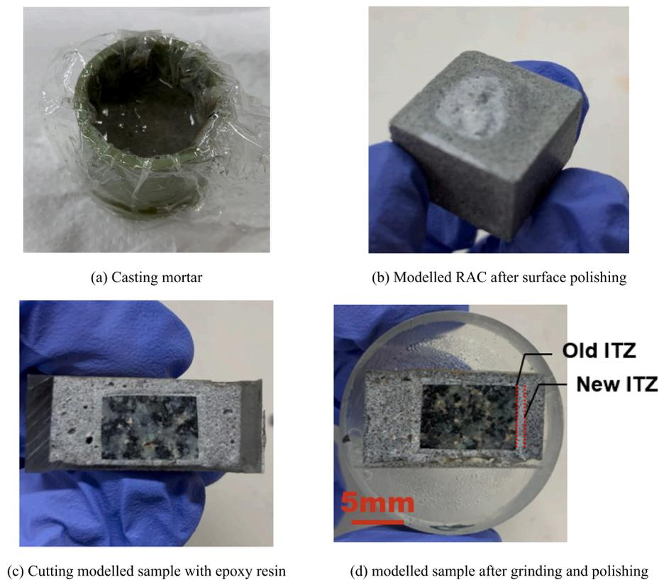
Fig. 4. Preparation of modelled recycled aggregate concrete.
