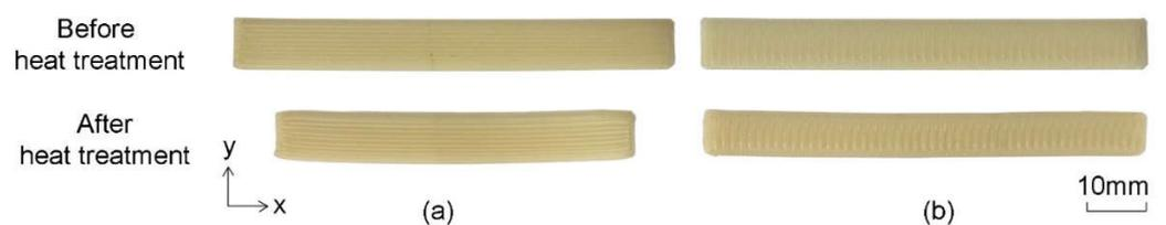
Figure 8. Comparison of the ABS specimens before and after the heat treatment: (a) 0° printing pattern; (b) 90° printing pattern.
