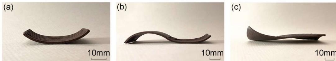
**Figure 10.** Final transformed shapes of 4D-printed WPC objects: (a) the concave design; (b) the wave design; (c) the spiral design.
