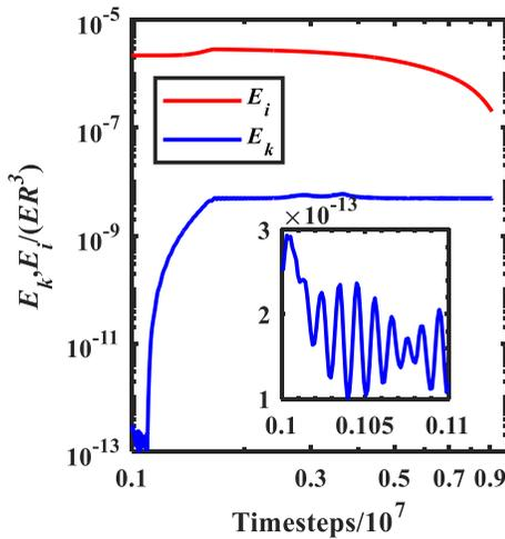
**Figure C3.** Energy evolution after completion of the pure normal compression process.  $E_i$  and  $E_k$  are internal and kinetic energies, respectively.
