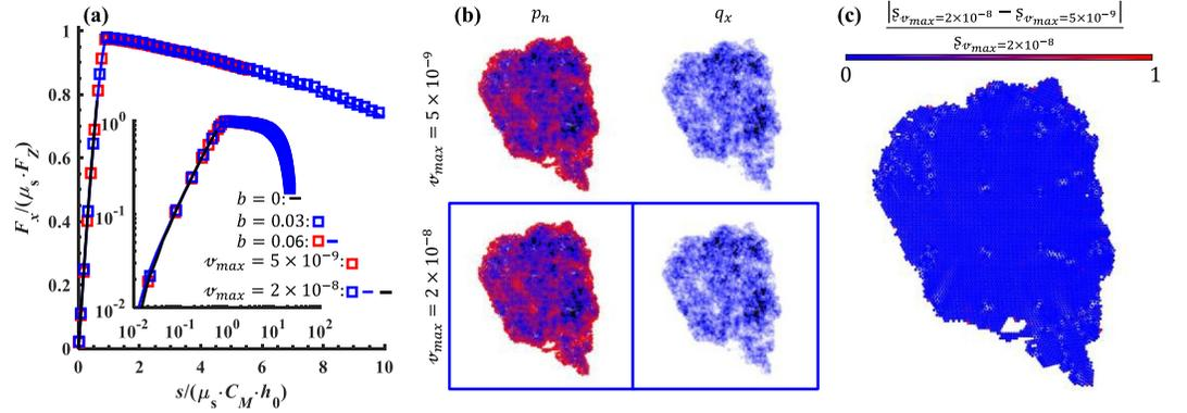
**Figure C2.** Convergence studies of applied normalized maximum velocity ( $v_{\max}$ ) by  $\frac{R}{\Delta t}$  and linear damping parameter, where  $\Delta t$  means the length of constant timestep; (b) Comparison of the distributions of  $p_n$  and  $q_x$  at  $s/(\mu_s \cdot C_M \cdot h_0) = 1$  between different  $v_{\max}$ ; and (c) Error in local partial-slide denoted by friction saturation induced by different  $v_{\max}$ .
