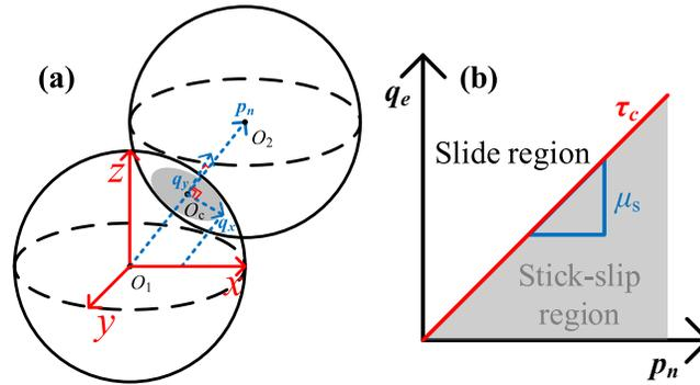
**Figure C4.** (a) Definitions of the local contact directions on or perpendicular to the contact plane; (b) The definition of the dry Coulomb friction model.
