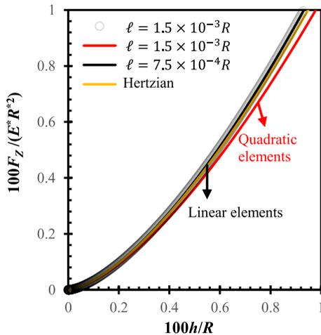
**Figure C1.** Comparisons of normal contact response (normalized normal contact force vs. normalized normal contact displacement) for the contact between an elastic sphere and a rigid planar surface between finite element method results of different mesh sizes and element types, referenced with the Hertzian contact solution.
