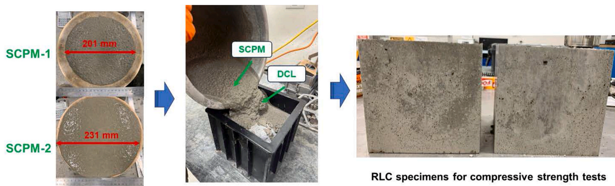
Fig. 2. Fabrication process of RLC specimens.
