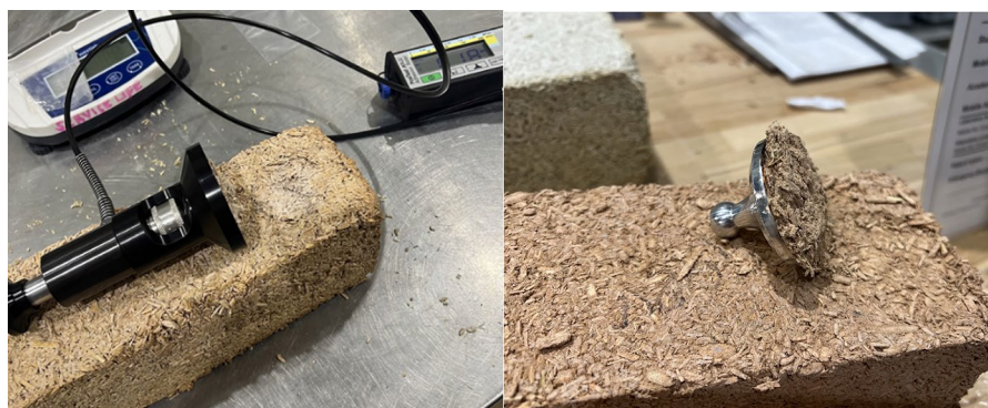
Fig. 5 Adhesion tester details: a The hydraulic pump with digital screen. b A dolly after failure
